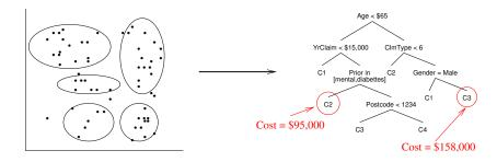
Working from left to right, we start with a dataset (a 2 dimensional dataset in this case) that has no specific target variables. Thus we have an unsupervised learning problem. By clustering the data in some way, for example using traditional k-means, we can end up with a collection of clusters. For a very large dataset (e.g., millions of entities) we may indeed end up with quite a number of clusters (upwards of 100 or even 1000).
